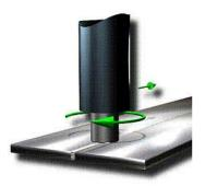
Friction Stir Welding (FSW)
